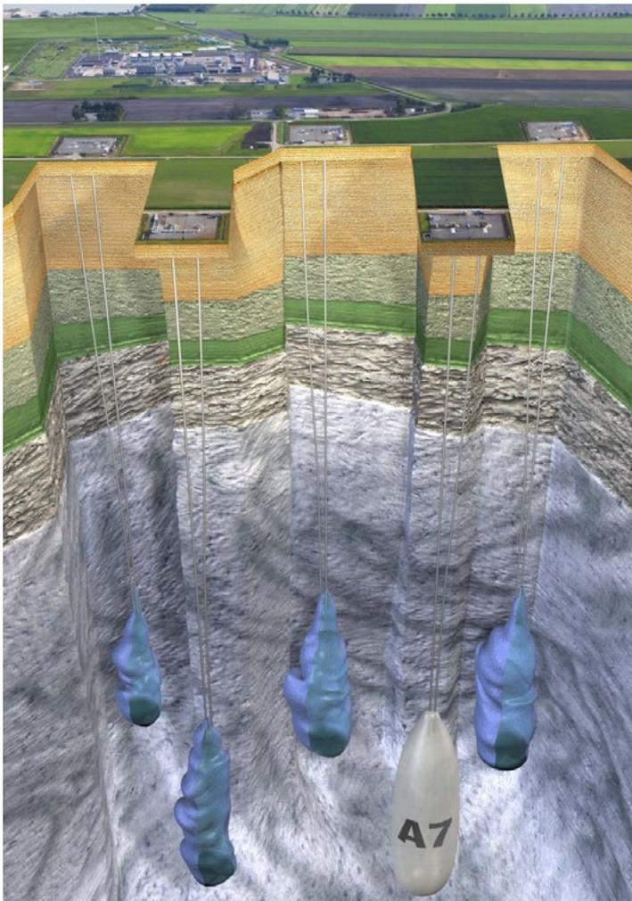
Dutch gas grid operator Gasunie is planning to develop its first large-scale hydrogen storage site at HyStock, Zuidwending. Here its subsidiary Energystock operates a storage facility with six underground salt caverns, which are currently used for storing natural gas. Four new caverns will be developed for hydrogen, with a total storage capacity of 20,000 tonnes.
