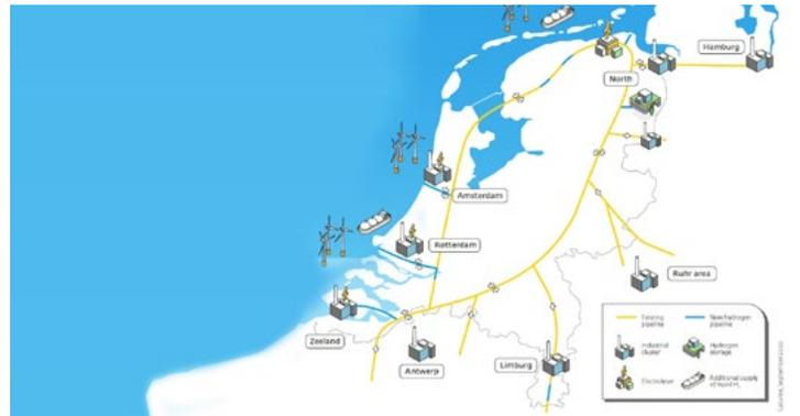
A national hydrogen backbone is being developed in the Netherlands, which will consist of 1,400 km of pipeline by 2030. The network will connect regional backbones with each other, with large clusters of industrial consumers and port facilities, as well as with storage facilities and grids outside the Netherlands. 85% of the backbone is expected to consist of reused gas infrastructure.
